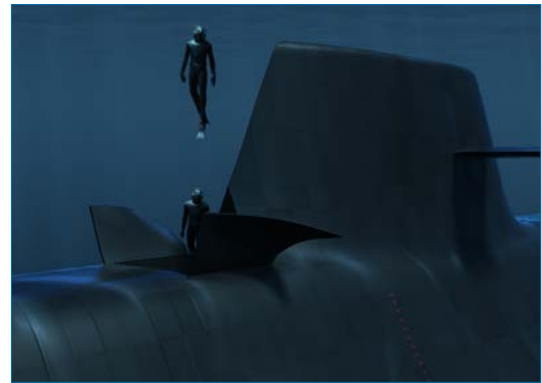
Special Forces divers exit from LLO chamber through concealed hatch
